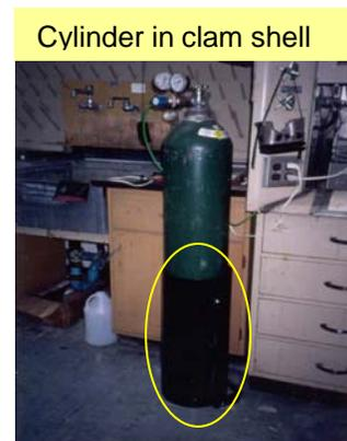
**Note:** For all *small gas cylinders* and specifically for those which require to be placed within the fume hood, use a frame casing (similar to clam shell) as shown in the pictures below:
