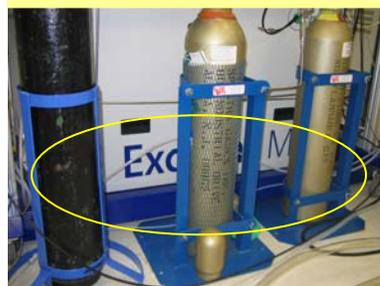
10. Cylinders should not be exposed to excessive dampness, or to corrosive chemical or fumes.
